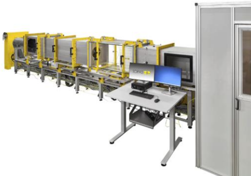
Test system ALF 114 for testing general air filters.
