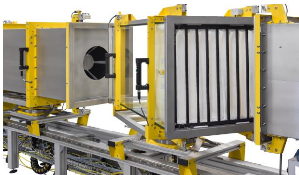
Rotatable and movable duct sections of the ALF114.
