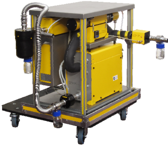
Blow-By Test Rig BBT 143 for measuring the oil concentration of blow-by gases: Gravimetric Measuring System GMS 141, Process Aerosol Photometer PAP 610 and PAP 612
