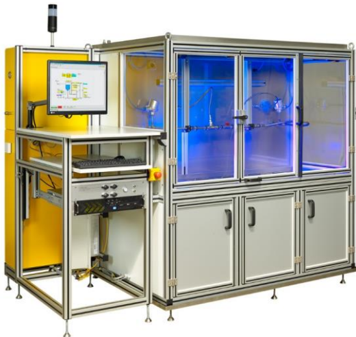
Diesel filter differential pressure test system LDP 190
